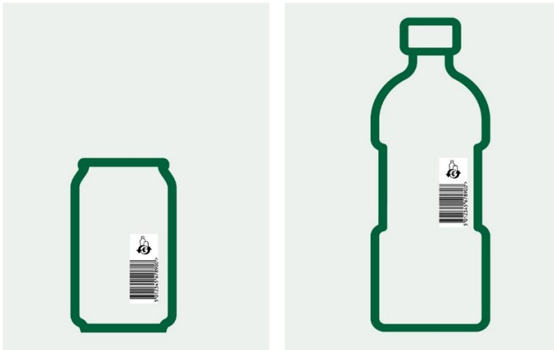
Figure 5: Example of vertical placement of the EAN/UPC barcode and Deposit Symbol on can and bottle
